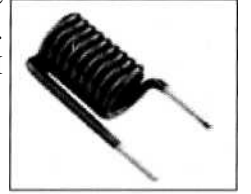
Figure 4.3: Air Core Inductors
